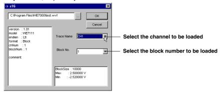
4. Click the [OK] button to load the arbitrary waveform data.
