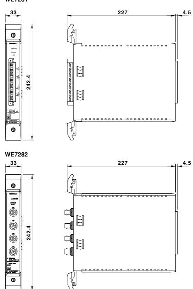
If not specified, the tolerance is  $\pm 3\%$ . However, in cases of less than 10 mm, the tolerance is  $\pm 0.3$  mm.
