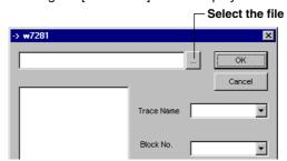
5. Clicking the button to the left of the [OK] button opens the [Open] dialog box. Select a file with extension [\*.wvf] or [\*.csv] and click the [Open] button.
