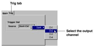
Click the [Source] button to select the source channel that will be used to output the trigger signal. When the output value of the source channel changes, the trigger signal is generated.
