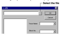
2. Clicking the button to the left of the [OK] button opens the [Open] dialog box. Select a file with extension [\*.wvf], [\*.csv], or [\*.s16] and click the [Open] button.
